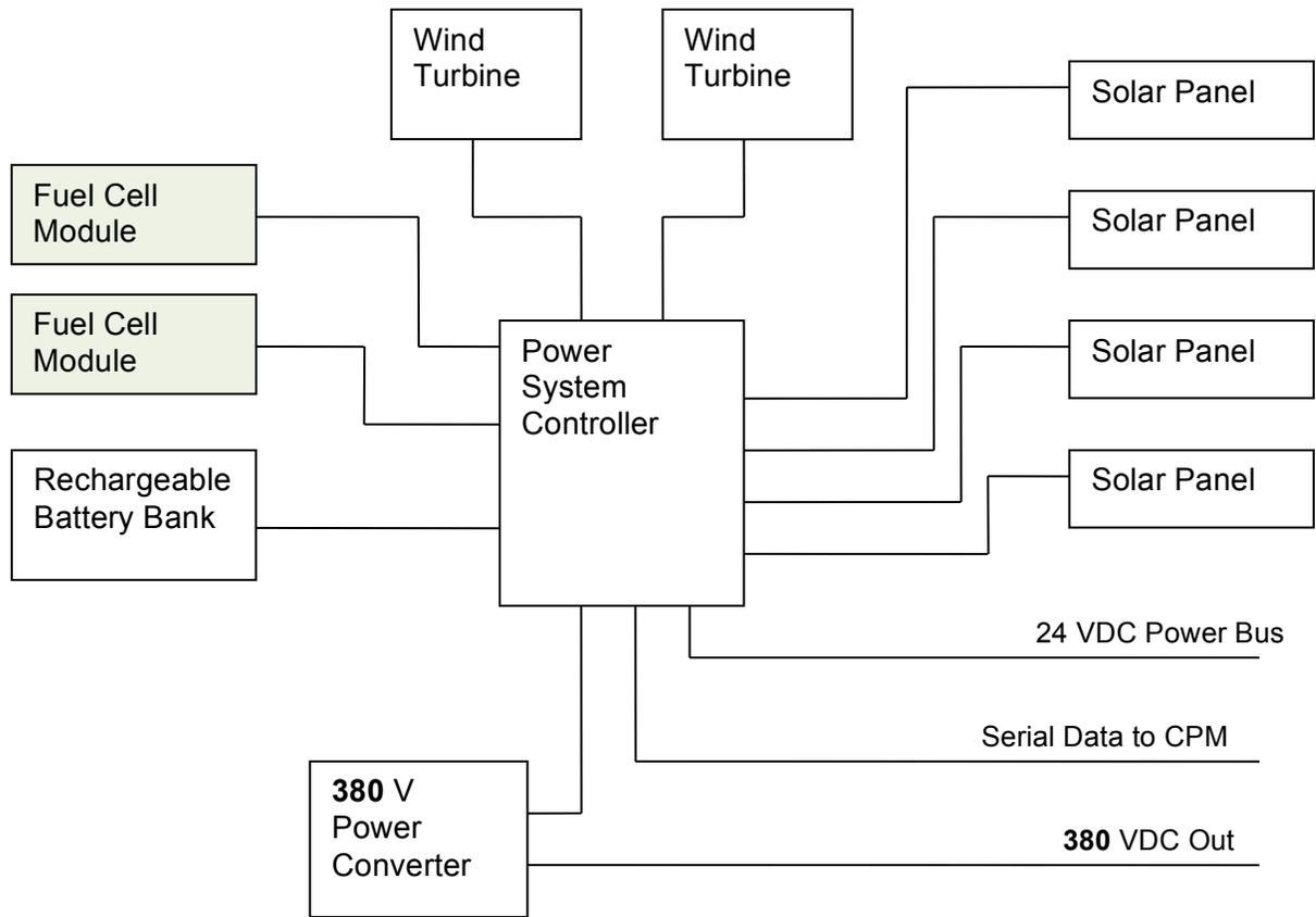
Fig. 1 – Block diagram of the Buoy Power System
