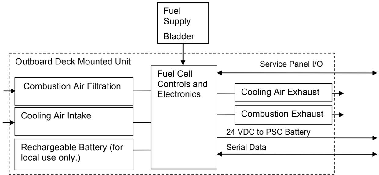
Fig. 2 – Block diagram of the Fuel Cell Module concept
